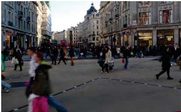
Unified paving to the entire crossing zone, which should be differentiated from pavement areas. Oxford Circus, London
